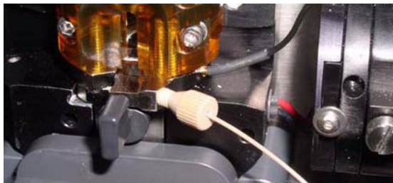
Figure 6-1 Closed-loop nozzle installed in flow cell
